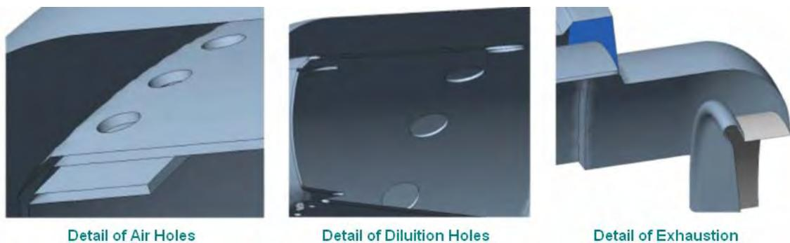
Figure 6 – Geometry Details
